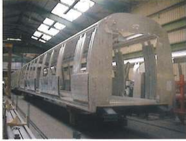
NEL Train Carbody Shell fabricated from aluminium with extrusion technique at Alstom Manufacturing Plant in Valenciennes, France on 13 September 2000.
