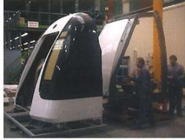
Assembly of Detrainment Door onto Electric Train End Mask at Alstom Manufacturing Plant in Valenciennes, France on 14 September 2000.
